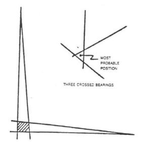
RIGHT ANGLE CROSSED BEARINGS, FIVE DEGREE READING ERROR
