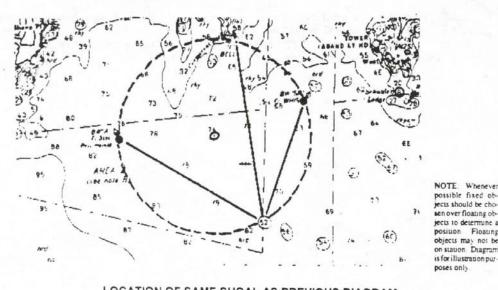
LOCATION OF SAME SHOAL AS PREVIOUS DIAGRAM, BUT WITH IMPROPER CHOICE OF OBJECTS. LOCATION IS INDETERMINATE.
